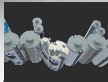
Double/double/single-diameter cylinder perfecting mechanism used on 8- to 10-color convertible perfecters
