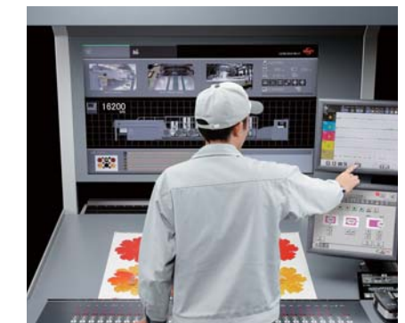
Press Information Display and easy-to-use touch panel display
