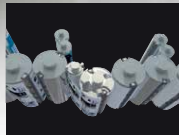
Double/double/single-diameter cylinder perfecting mechanism used on 8- to 10-color convertible perfectors
