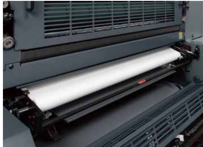
Automatic blanket cleaning device
