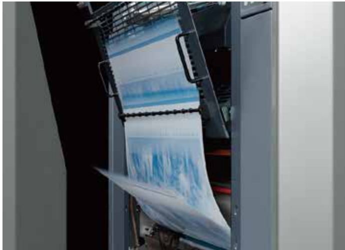
SPC Semiautomatic Plate Changing System
