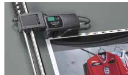
Printing density control system PDS-E SpectroJet
