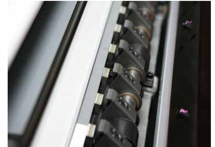
Double sprung gripper mechanism employing torsion bars
