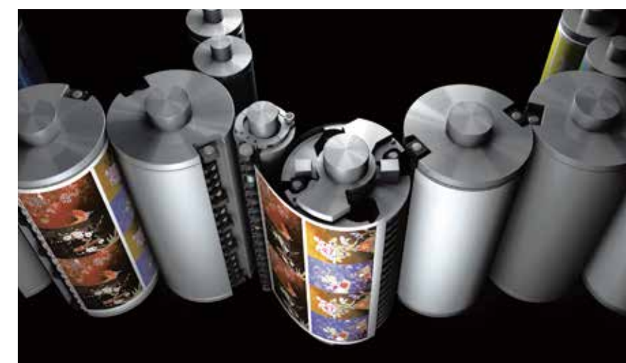
Double/double/single-diameter cylinder perfecting mechanism*
