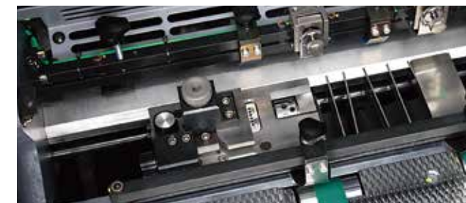
Pneumatic side lay device
