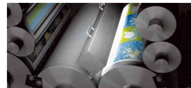
Inter-deck UV curing unit over the impression cylinder
